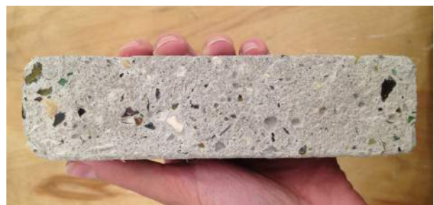
EConcrete designed to promote biological assemblages using recycled materials from the SIMS glass facility. Developed by SeARC Consulting in conjunction with SCAPE/LANDSCAPE ARCHITECTURE PLLC.
